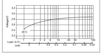
Capacity vs. load resistance
